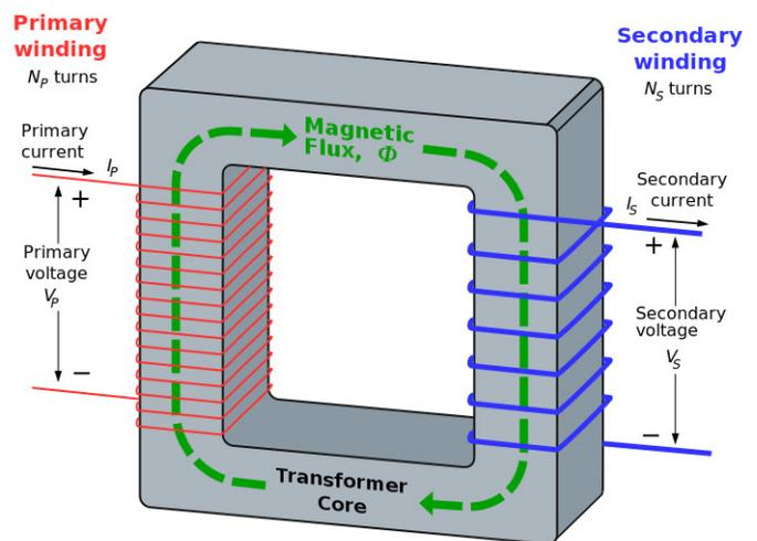
*Power ( $VI$ ) applied to the primary coil is magnetically transferred to the secondary coil, hence the galvanic isolation.*
