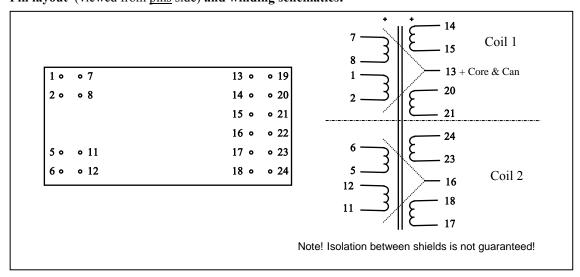
**Spacing between pins:** 5.08 mm (0.2")
