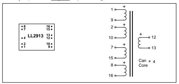
**Spacing between pins:** 2.54 mm (0.1") **Spacing between rows of pins:** 22.86 mm (0.9")
