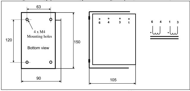
Weight:4.9 kgStatic resistance of each winding: $0.05 \Omega$ Isolation between windings / between windings and core:4 kV / 2 kV
