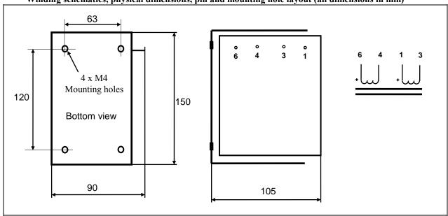
Weight: 4.9 kg 5.6 Ω Static resistance of each winding:
