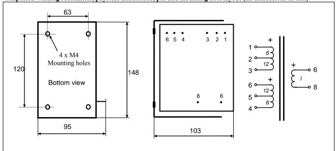
Weight: 4.6 kg Static resistance of each primary:  $82 \Omega$ **Static resistance of secondary:**  $0.1 \Omega$ Isolation between windings / between windings and core: 4 kV / 2 kV Max DC current through any primary winding (10W heat dissip): 350 mA
