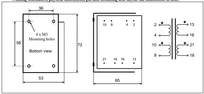
Weight: $0.6 \, \mathrm{kg}$ Static resistance of each primary: $7 \, \Omega$ Static resistance of secondary: $7 \, \Omega$
