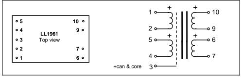
**Dimensions** (L x W x H above PCB, in mm) 44 x 30 x 23 5.08 mm (0.2") Spacing between pins Spacing between rows of pins 30.48 mm (1.2") Rec. PCB hole diameter: 1.5 mm Weight: 93 g Static resistance of each primary:  $1.2 \Omega$ Static resistance of each secondary:  $6.4 \Omega$ -1 dB at 12Hz Frequency response, serial-serial connection (source 50  $\Omega$ , load 330k $\Omega$ , relative to 1kHz) -1 dB at 100kHz Isolation between windings/ between windings and core: 3 kV / 1.5 kV
