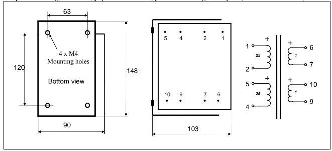
Weight: 4.6 kg  $112 \Omega$ Static resistance of each primary:  $0.3 \Omega$ Static resistance of each secondary: 4 kV / 2 kV Isolation between windings / between windings and core: Max DC current through any primary winding (10W heat dissip): 210mA
