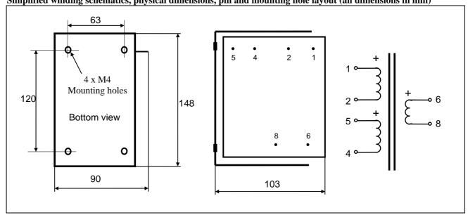
Weight: 4.6 kg Static resistance of each primary:  $260 \Omega$ **Static resistance of secondary:**  $0.3 \Omega$ Isolation between windings / between windings and core: 4 kV / 2 kV Max DC current through any primary winding (10W heat dissip): 140mA
