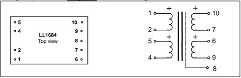
**Dimensions** (L x W x H above PCB, in mm) 42 x 28 x 22 5.08 mm (0.2") Spacing between pins 30.5 mm (1.2") Spacing between rows of pins Rec. PCB hole diameter: 1.5 mm Weight: 81 g **Static resistance of each primary:**  $41\Omega$ Static resistance of each secondary:  $41\Omega$ Distortion + 23 dBU 0.1% @ 50 Hz (primaries connected in series,
