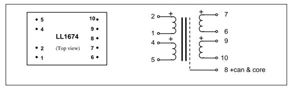
**Spacing between pins:** 5.08 mm (0.2") **Spacing between rows of pins:** 30.48mm (1.2")
