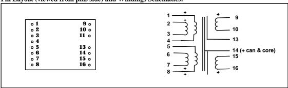
2.54 mm (0.1") Spacing between pins: **Spacing between rows of pins:** 22.86 mm (0.9")
