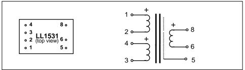
Spacing between pins:3.81 mm (0.15")Spacing between rows of pins:20.32 mm (0.8")Weight:25 g
